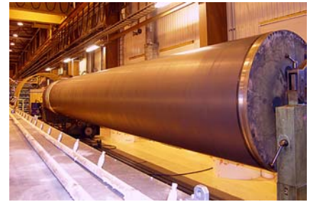
Fig. 4 Paper machine center press roll with a thermally sprayed ceramic coating (Metso Paper Inc.)
