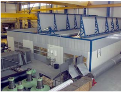
Fig. 2 Thermal spray booths for coating of paper machine rolls (AK-Tehdas Oy)
