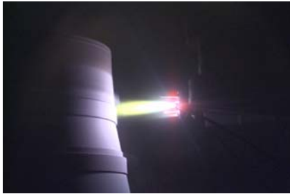
Fig. 5 Plasma spraying of gas turbine components at Volvo Aero Corp.
